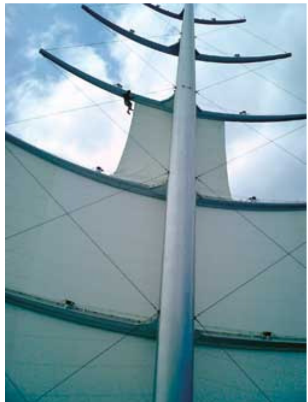
Figure 3: In mast furling, with one of the crew inspecting the initial set-up. Photograph courtesy of Insensys.
