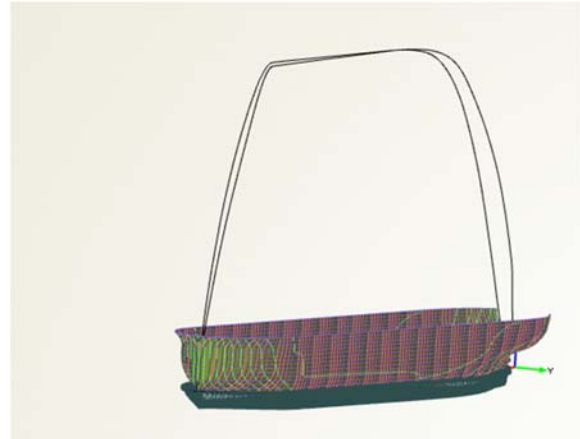
Picture [1]: Finalized hullform after Lackenby variation
