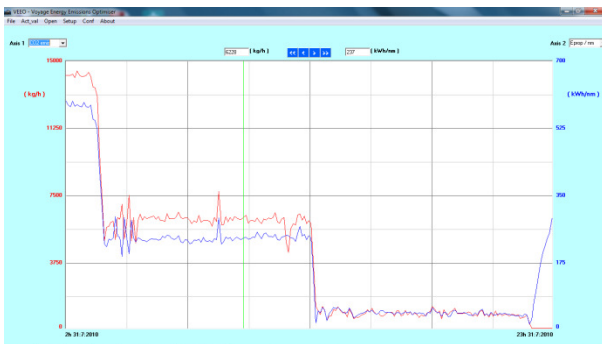
Figure 8 - CO 2 (kg/h) & Propulsion Energy per nm as a function of time.
