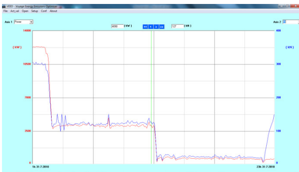
Figure 7: Main engine shaft power & Hull resistance versus time.
